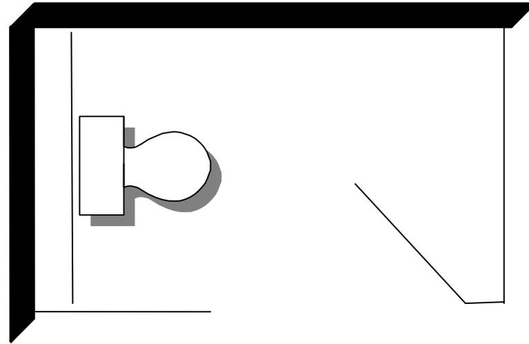
SINGLE IN LINE PARTITION CUBICLES SHOWING IPS AT THE BACK
